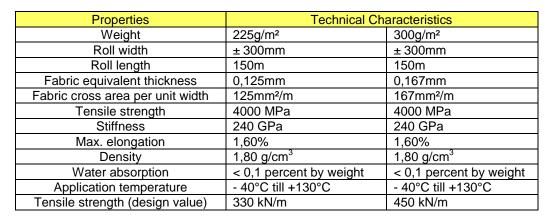
The above values are typical and indicative only. The achievable properties obtained from tensile tests are dependant on the impregnating/laminating resin used and the type of tensile testing procedure. Apply material reduction factors according to the relevant design standard.
